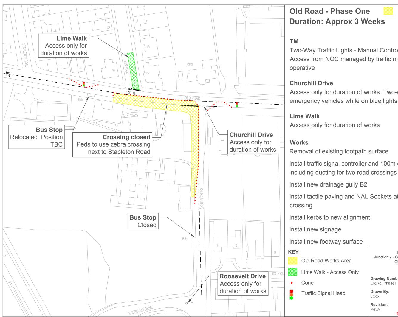
Two-Way Traffic Lights - Manual Control 7AM - 8PM. Access from NOC managed by traffic management
